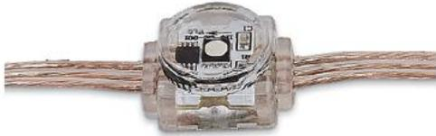
D115-S1-RGB is designed for high-end decoration. It adopts 1pcs high brightness SMD3535 LEDs, round-shaped completely waterproof design with IP rate IP66. It is easy and reliable to install, of high flexibility of connection. It can be applicable for any curves or heteromorphic facade.
