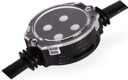
D132-S4-RGB is designed for high-end decoration. It adopts 4pcs high brightness SMD3535 LEDs, round-shaped completely waterproof design with IP rate IP66. It is easy and reliable to install, of high flexibility of connection. It can be applicable for any curves or heteromorphic facade.
